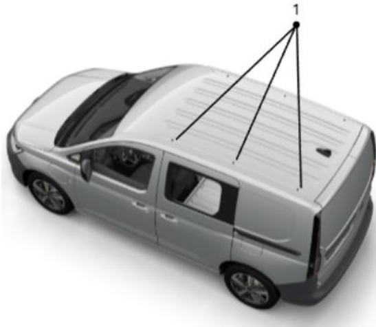
Fig. 1: Caddy mounting points
