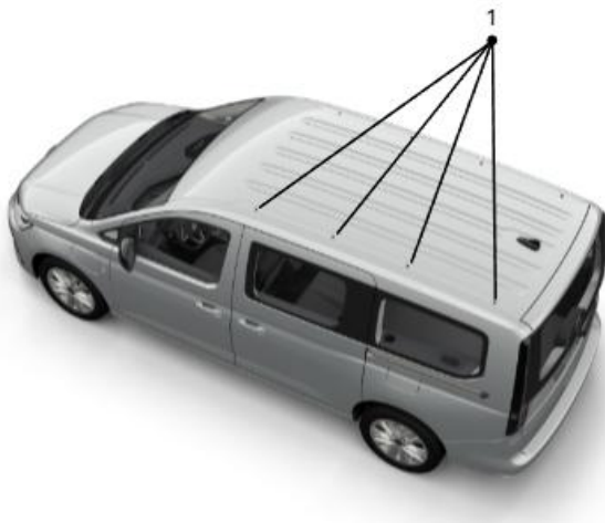
Fig. 2 Caddy Maxi mounting points
