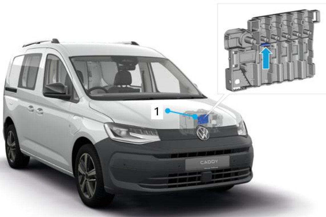
Fig. 3: Location of the second battery preparation on the main fuse box
