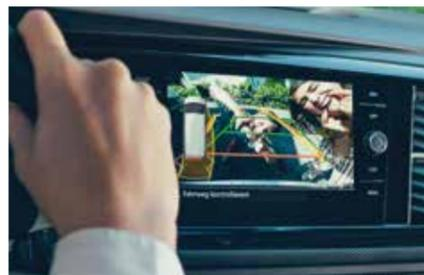
**Rear Assist 顯影式停車導引系統**
